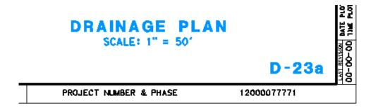
Note: A <u>lowercase</u> letter is used in the name of the MicroStation design file, TIFF file, Sheet ID and the sheet numbers in the Project Identification Block when revised or additional sheet are added to the As-Built plans. During the addendum process (which is prior to contract award), an <u>uppercase</u> letter is used in the Sheet ID when a sheet is added (see the Ready To List and Construction Contract Award Guide - RTL Guide).
