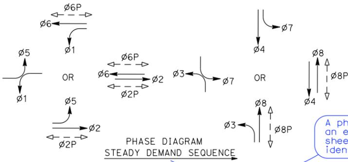
A phase diagram presented on an electrical systems plan sheet does not need to be identified as "NO SCALE."
