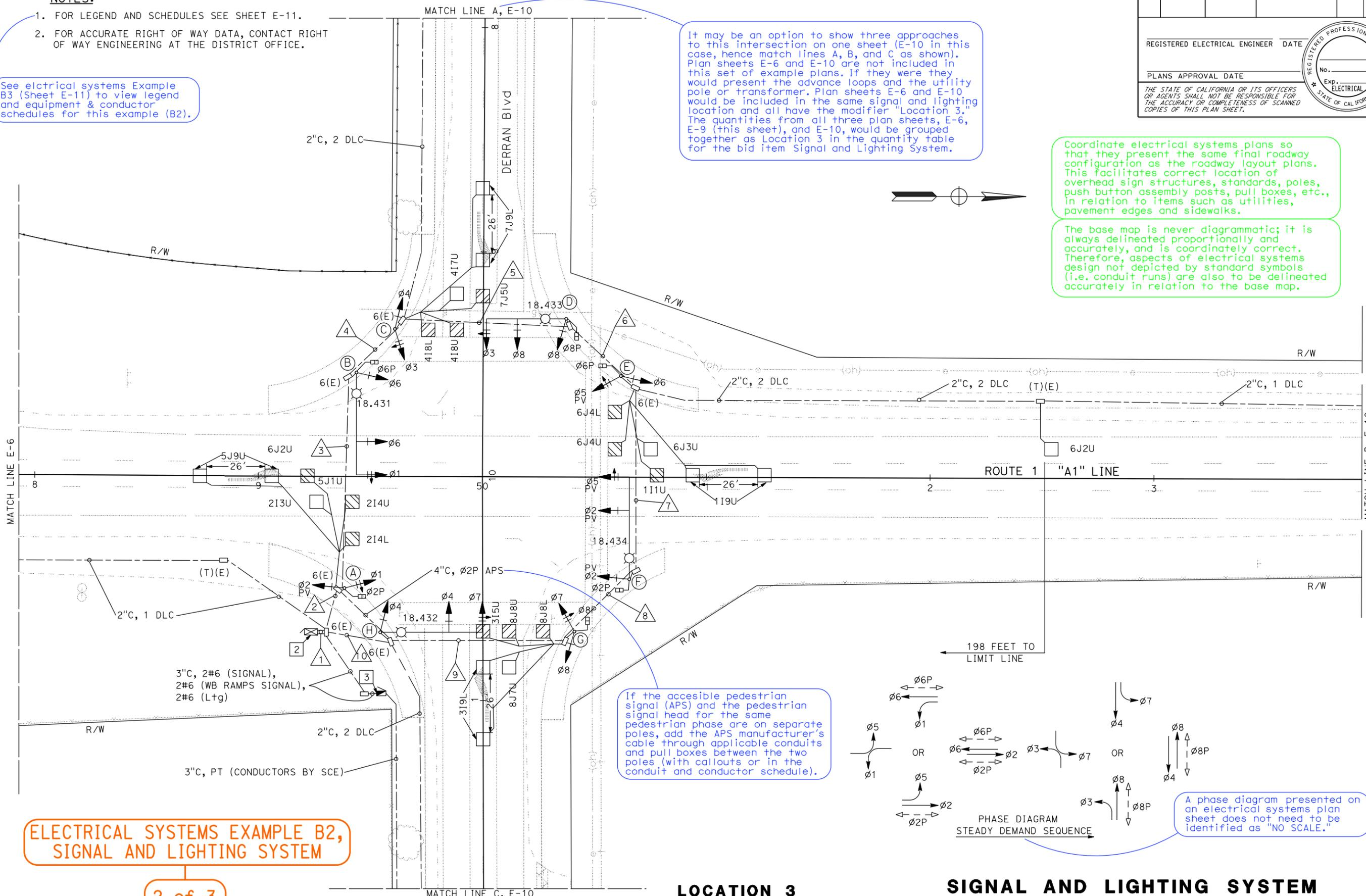
If the accessible pedestrian signal (APS) and the pedestrian signal head for the same pedestrian phase are on separate poles, add the APS manufacturer's cable through applicable conduits and pull boxes between the two poles (with callouts or in the conduit and conductor schedule).
