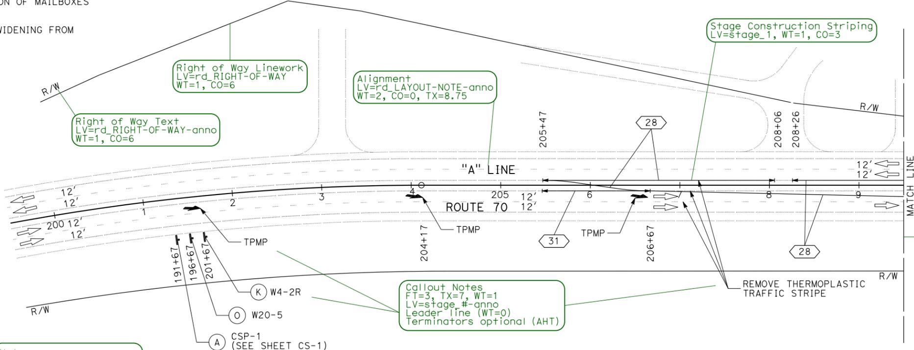
Stage Construction work Level = "Stage\_#", Weight=1, Color=Varies on Stage Number
