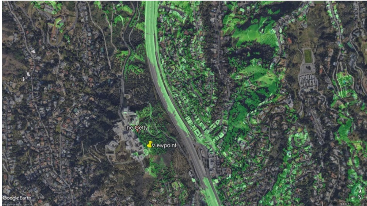
Figure D-1: Google Earth Pro delineation of a project viewshed (shown in green)
