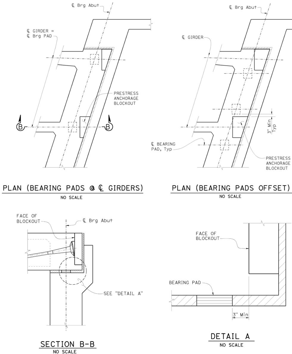
**Figure 6.6.1 Bearing Pad Location at Anchorage Blockout**
