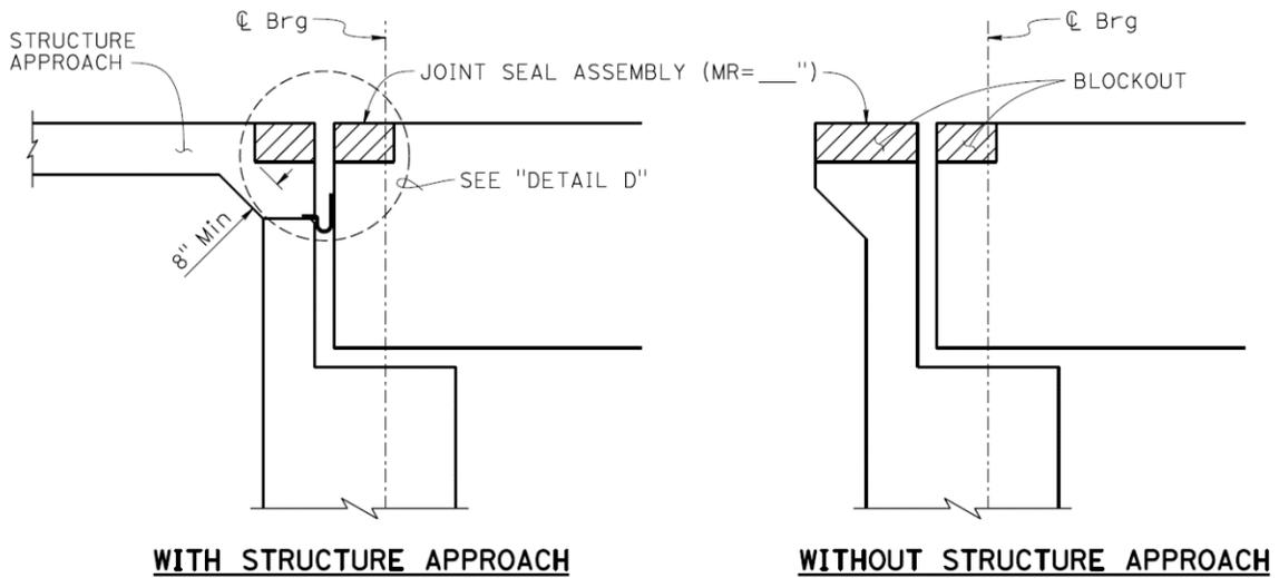
**Figure 6.7.2 Joint Seal Assemblies (MR > 2 1/2'')**
