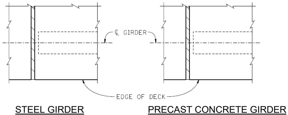
**Figure 9.5.1 Deck Joints at Girders (No Skew)**
