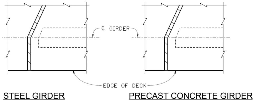
**Figure 9.5.3 Deck Joints at Girders (Over 20° Skew)**
