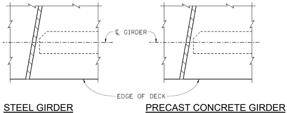
**Figure 9.5.2 Deck Joints at Girders (Skew 0° to 20°)**
