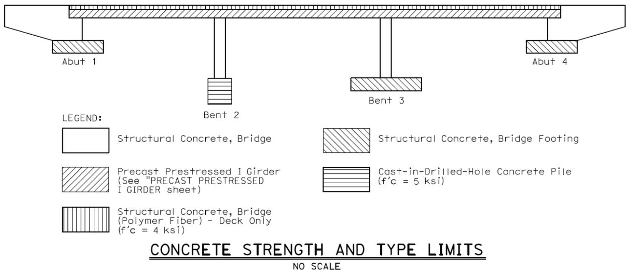
**Figure 9.8.1 Concrete Strength and Type Limits Diagram
