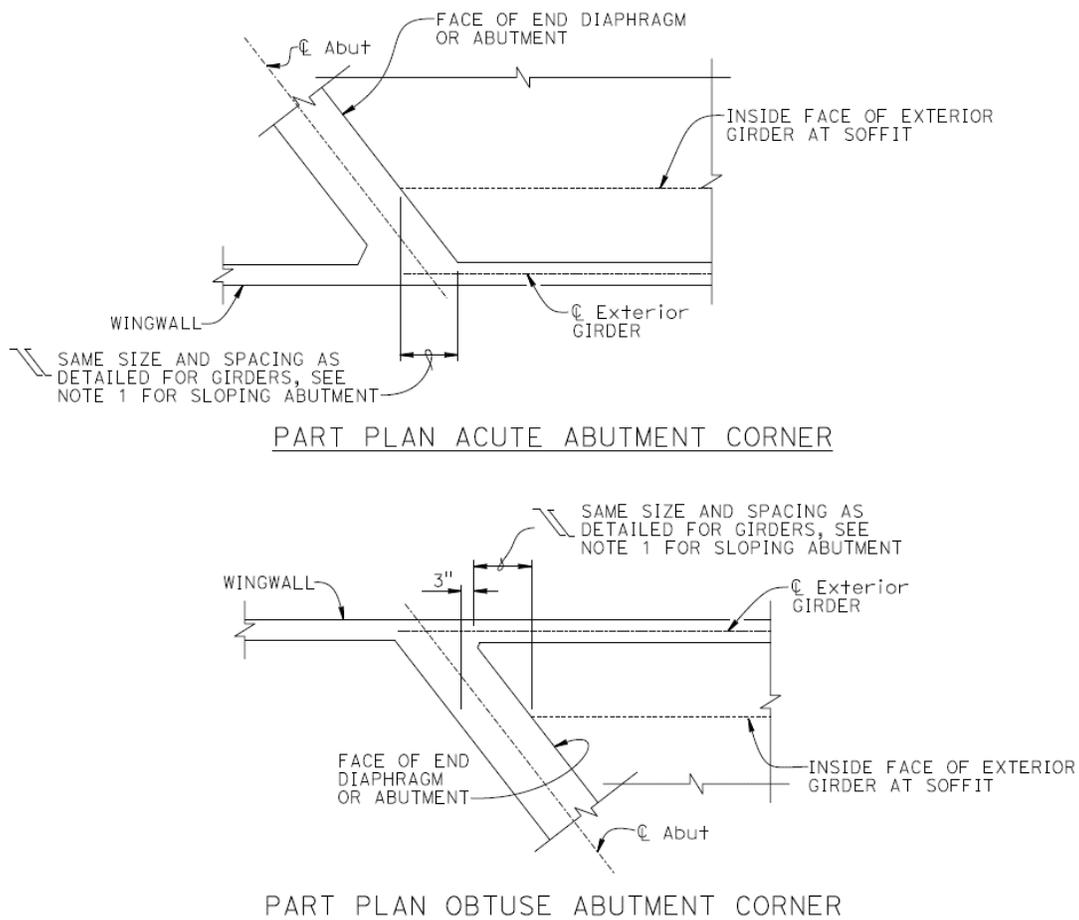
**Figure 9.6.1 Stirrup Reinforcement at Abutments (Sloping Exterior Girder)**
