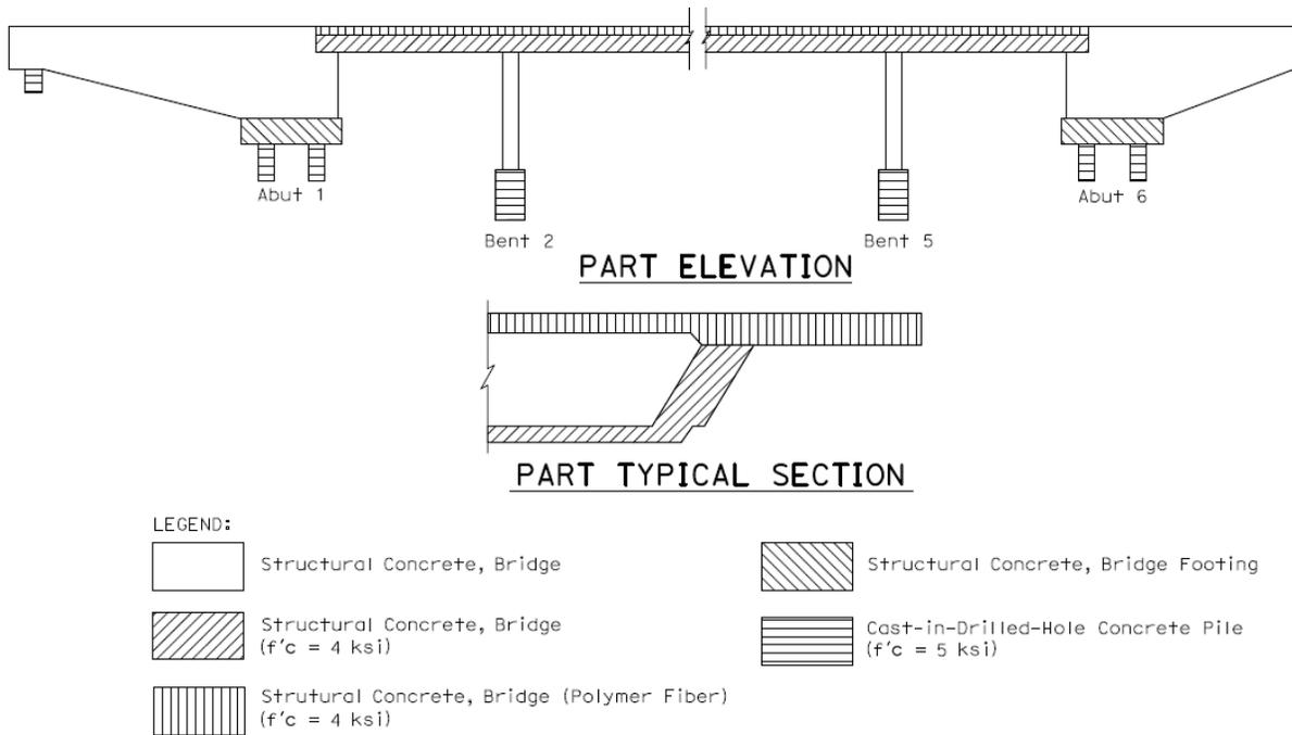
**CONCRETE STRENGTH AND TYPE LIMITS**
