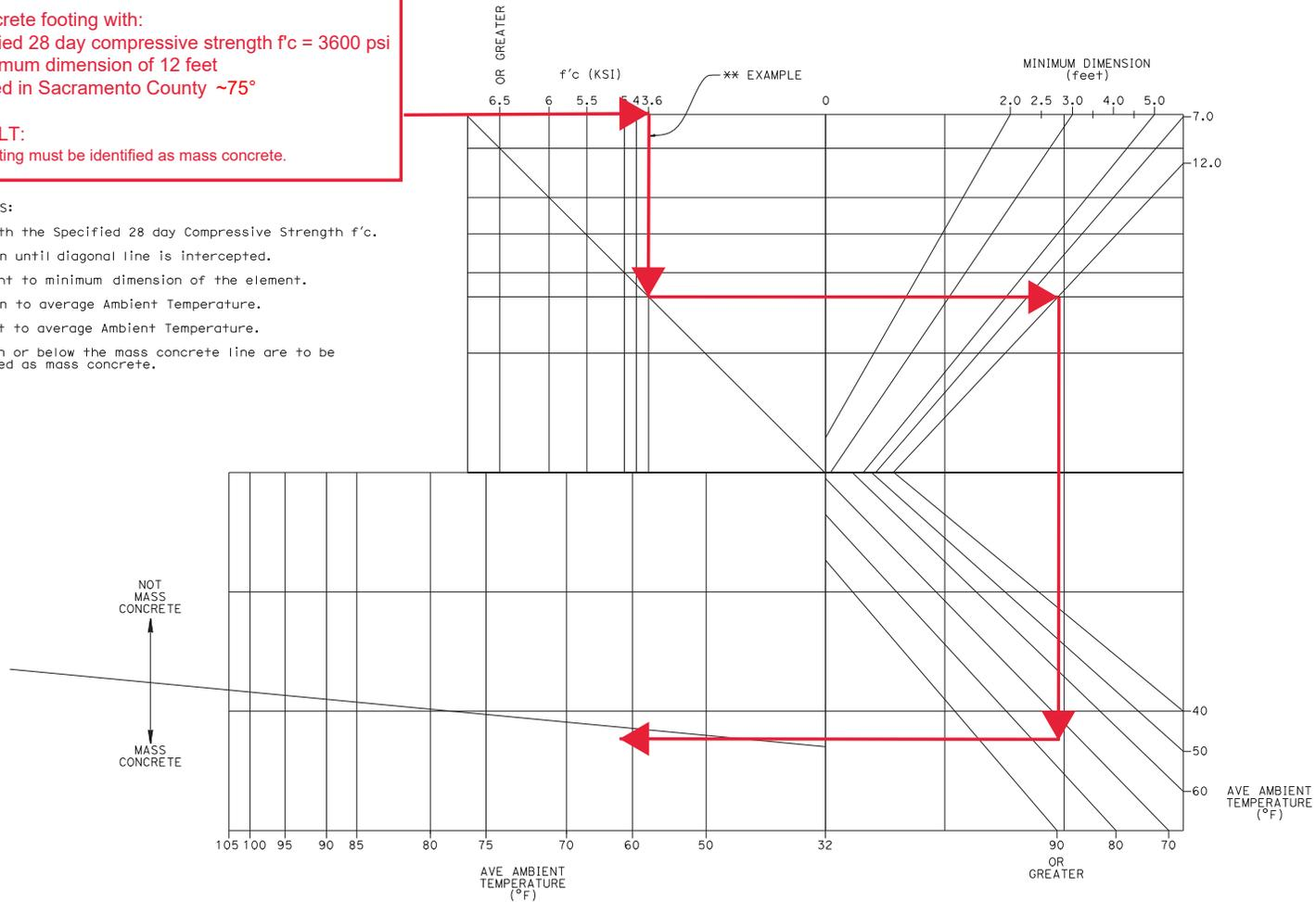
**Figure 5.13.2.1 Mass Concrete Prediction Nomogram - Example**
