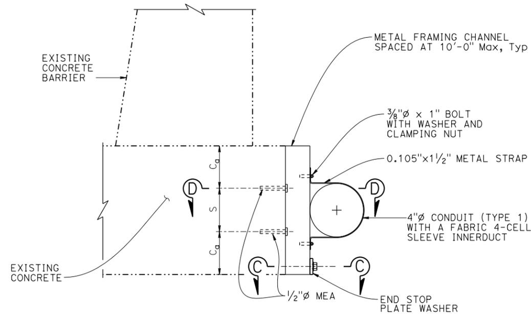
**ATTACHMENT TO SLAB OR CULVERT DETAIL**
