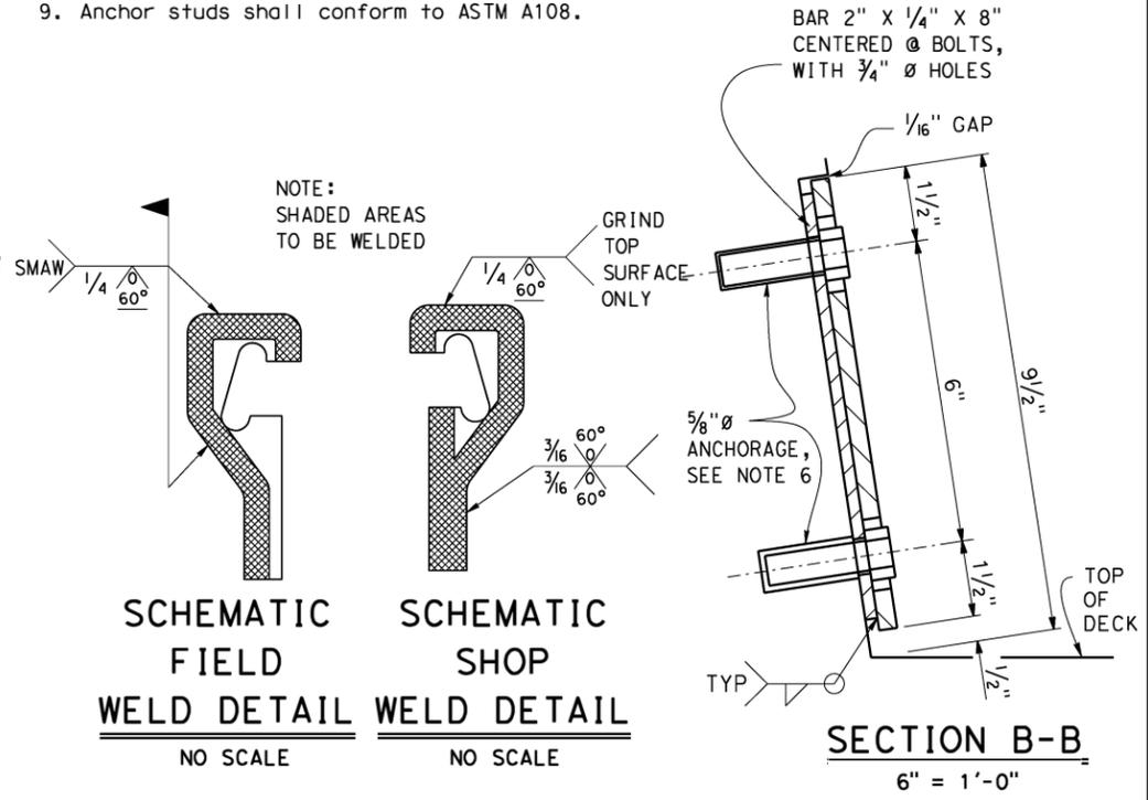
**SCHEMATIC FIELD WELD DETAIL**
