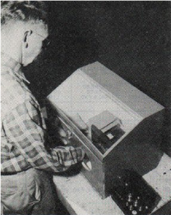
FIGURE 7 WEIGHING PADS – NOTE PAD STACK INSIDE BOX
