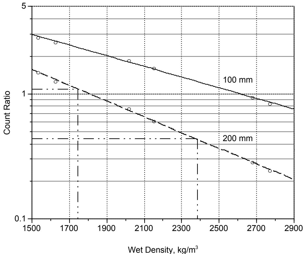
Density versus Count Ratio on Six Standard Blocks
