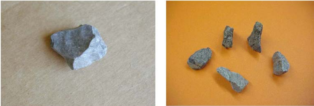
Figure 2. Crushed Particles (Fractured face is greater than 25 % of largest cross-sectional area of the aggregate)
