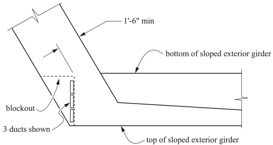
Plan View of Skewed Abutment Diaphragm with sloped exterior girder
