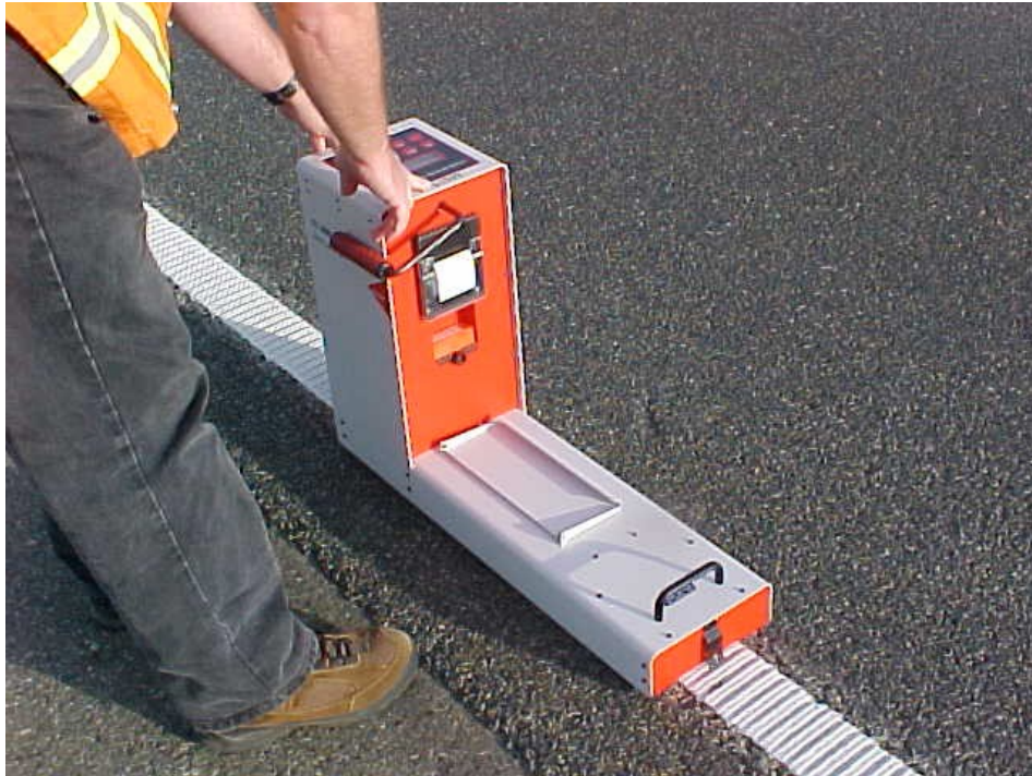
Photo 3: Traffic striping SSPs now require minimum levels of stripe retro reflectivity (nighttime visibility) for new striping. The Chemical Testing Branch measuring the retro reflectivity of questionable new striping.
