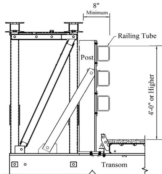
Figure 17.1.3 Vehicular Railing Offset Requirement for Railing Height of 4 feet
