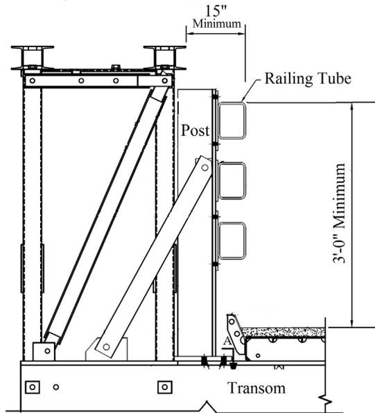
Figure 17.1.2 Vehicular Railing Offset Requirement for Railing Height of 3 feet
