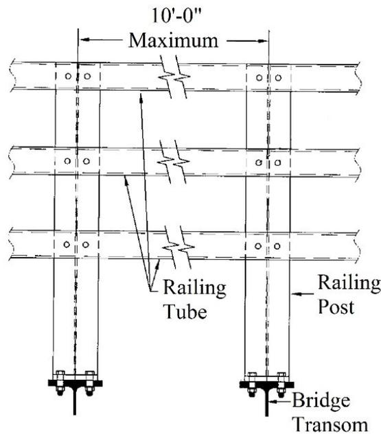
Figure 17.1.1 Vehicular Railing Elevation
