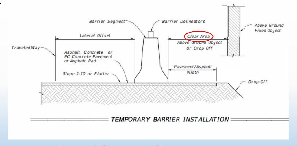
Clear area = dynamic deflection plus rollover Rollover clear area measured from traffic face less the system width
