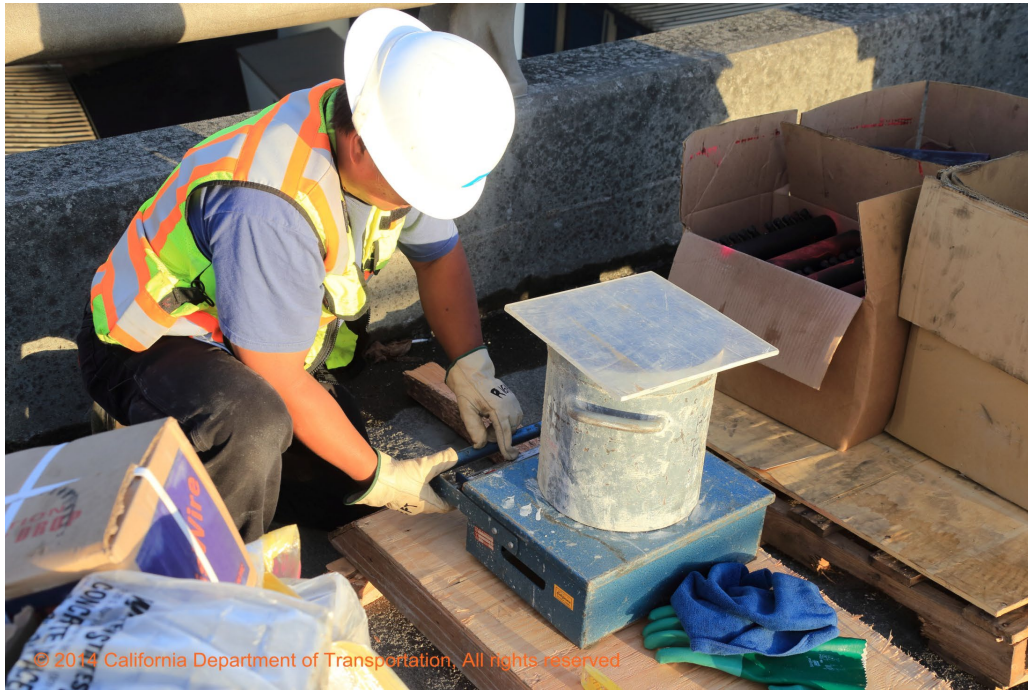
Figure 5. Concrete unit weight test
