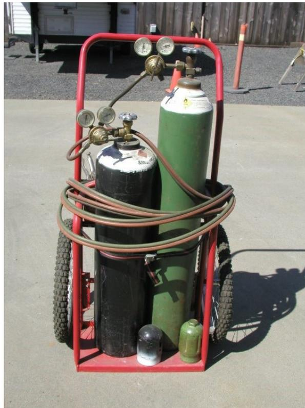
Figure 3-10. Oxyacetylene Torch Setup
