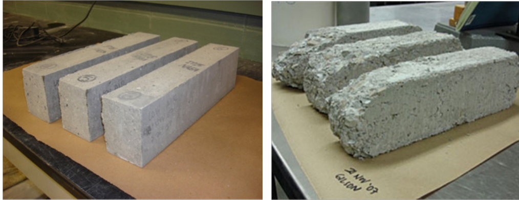
Figure 1-6. Freeze-Thaw Damage, Before and After Photos 3 .
