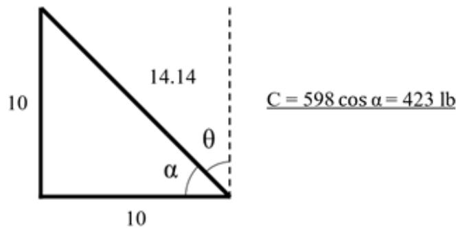
Figure D-17-7. Geometric Components of Compression Strength Value for Bracing (A) Middle Tier
