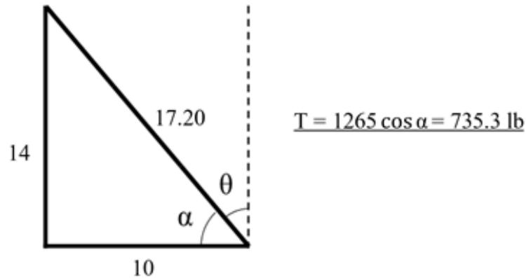
**Figure D-17-12. Geometric Components of Tension Strength Value for Bracing ②
