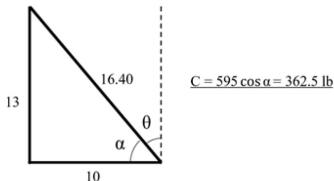
**Figure D-17-10. Geometric Components of Compression Strength Value for Bracing**
