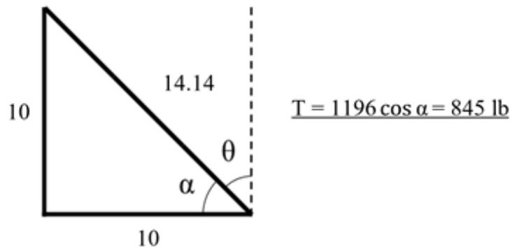
**Figure D-17-6. Geometric Components of Tension Strength Value for Bracing (A)
