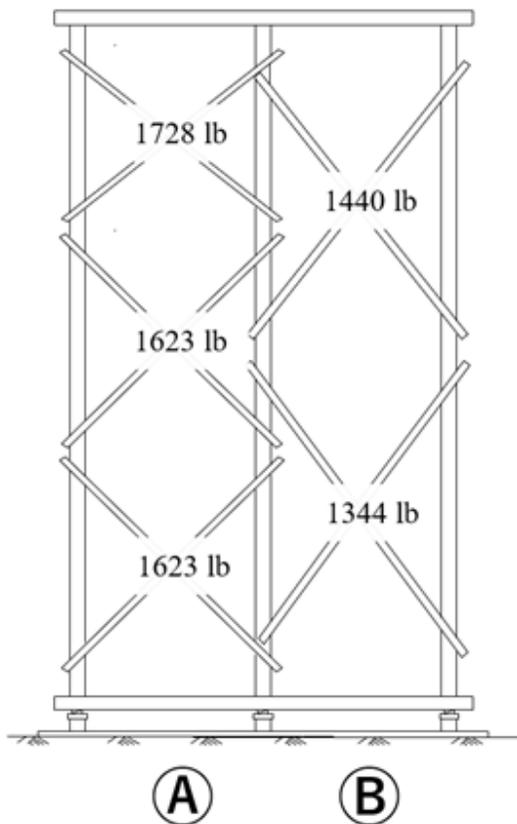
The total resisting capacity of the bracing = the sum of the weaker pair of braces in A and the weaker pair of braces in B.
