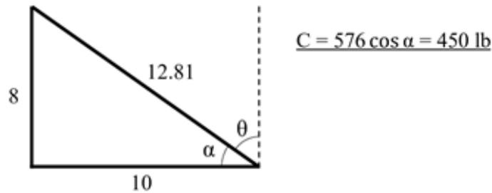
Figure D-17-4. Geometric Components of Compression Strength Value for Bracing
