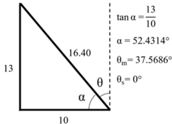
**Figure D-17-8. Bracing B Top Tier Member Lengths and Orientation**
