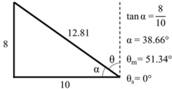
**Figure D-17-2. Bracing (A) Top Tier Member Lengths and Orientation**
