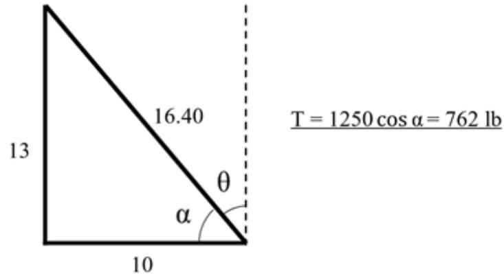
**Figure D-17-9. Geometric Components of Tension Strength Value for Bracing (B)
