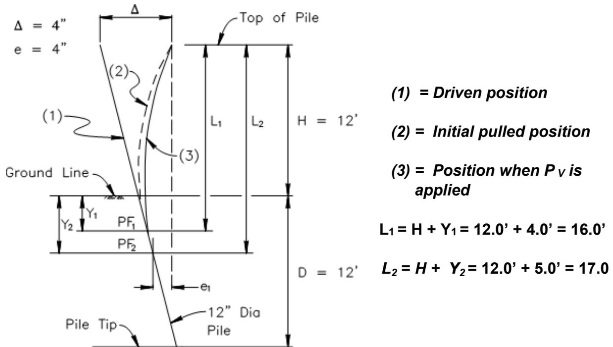
1. Calculate  $F_1$  = force to pull pile into line
