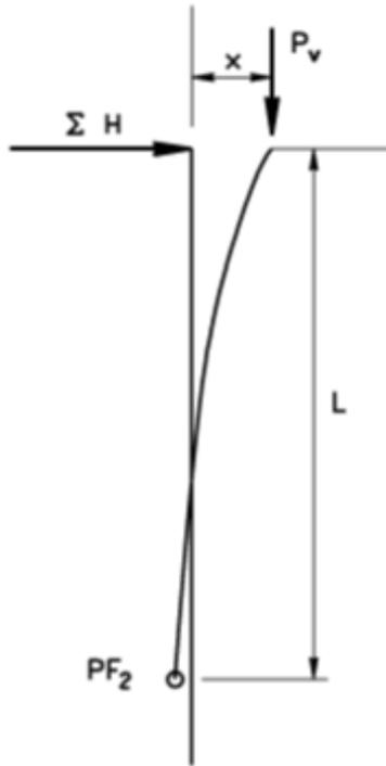
$X$  = displacement due to total H load
