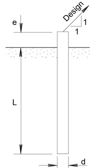
**Figure D-29-4. Pile Lateral Loading in Cohesive Soil**
