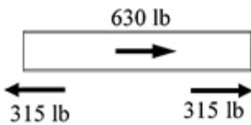
Half the horizontal design force for stringer AB is taken at stable bent A. Since the 315 lb is less than the FTC = 648 lb, no mechanical connection is required. The other half is strutted ahead through bent B.
