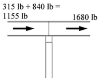
Since the FTC between bent C and Stringer CB = 864 lb < 1155 lb, and the FTC between bent C and stringer CD = 1728 lb > 1155 lb, a mechanical connection between bent C and stringer CB will be required, but friction between bent C and stringer CD will be adequate to strut the 1155 lb coming from spans AB & BC to a stable bent.
