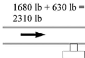
Since the FTC between bent H and stringer HG = 648 lb < 2310 lb, a mechanical connection is required to get the forces coming from spans EF, FG, & GH into the stable bent H.
