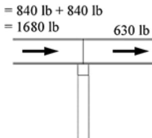
Since the FTC between bent G and stringer GF = 864 lb < 1680 lb, and since the FTC between bent G and stringer GH = 648 lb < 1680 lb, mechanical connections between both stringers (GF and GH) and bent G will be required to strut the forces to stable bent H.
