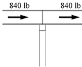
Since the FTC between bent F and stringer FE = 1728 lb > 840 lb, and since the FTC between bent F and stringer FG = 864 lb > 840 lb, the 840 lb coming from span FE can be strutted ahead to a stable bent and no mechanical connections are required.
