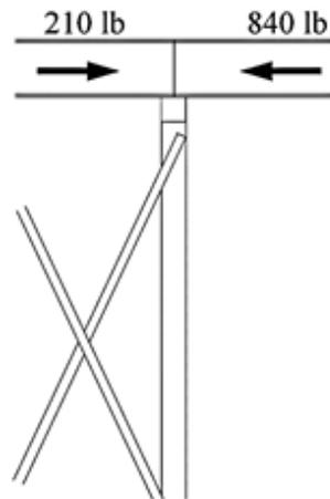
Since the FTC between bent E and stringer ED = 432 lb > 210lbs, the 210 lb can be taken to the stable bent E through friction. The 1680 lb in span EF will cause a reaction of 840 lb (at each end) and since the FTC between bent E and stringer EF = 1728 lb > 840lbs, the 840 lb can be taken to the stable bent E through friction and the diagonal bracing will then have to take 210 + 840 = 1050 lbs.
