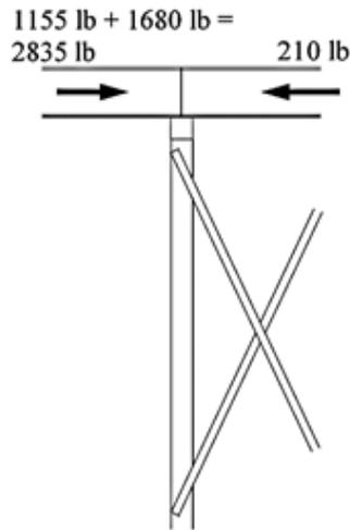
Since the FTC between bent D and stringer DC = 1728 lb < 2835 lb, a mechanical connection between bent D and stringer DC will be required.
