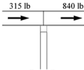
Since the FTC between bent B and stringer BA = 648 lb > 315 lb, and since the FTC between bent B and stringer BC = 864 lb > 315 lb, the 315 lb coming from span BA can be strutted ahead to a stable bent and no mechanical connections are required.
