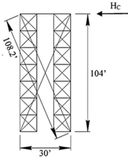
$$\text{Excess overturning, one tower} = 794^{\text{ft-k}} - 304^{\text{ft-k}} = 490^{\text{ft-k}}$$
