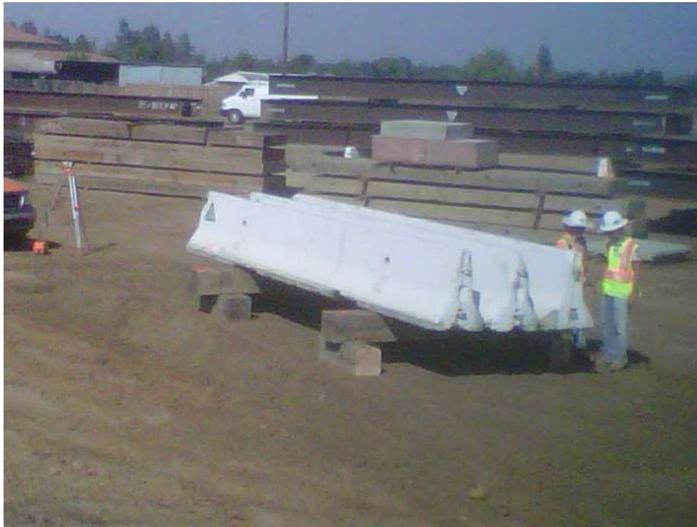
Figure 8-16. Simple Static Soil Load Test Using K-Rail.
