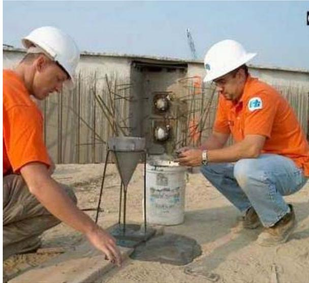
**Photo F-1 – Testing Efflux Time of Grout.**
