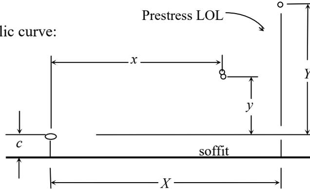
Example: Given the tendon profile shown below, find the equation to calculate y.
