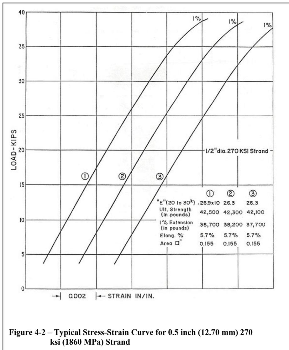
Figure 4-2 – Typical Stress-Strain Curve for 0.5 inch (12.70 mm) 270 ksi (1860 MPa) Strand
