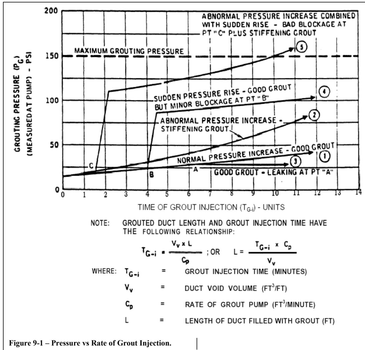
Figure 9-1 – Pressure vs Rate of Grout Injection.
