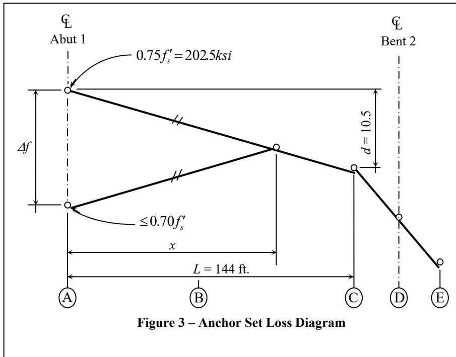
$$x = \sqrt{\frac{E(\Delta L)L}{d}} = \sqrt{\frac{(28,000\text{ksi})(0.375\text{in})(144\text{ft})}{(10.5\text{ksi})(12\text{in}/\text{ft})}} = 109.5\text{ft}$$
