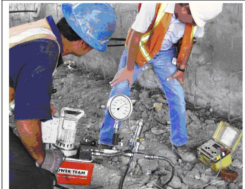
Photo B-2 – Model P-3500 Digital Display Strain Indicator.
