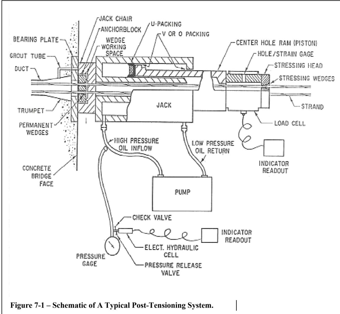
Figure 7-1 – Schematic of A Typical Post-Tensioning System.
