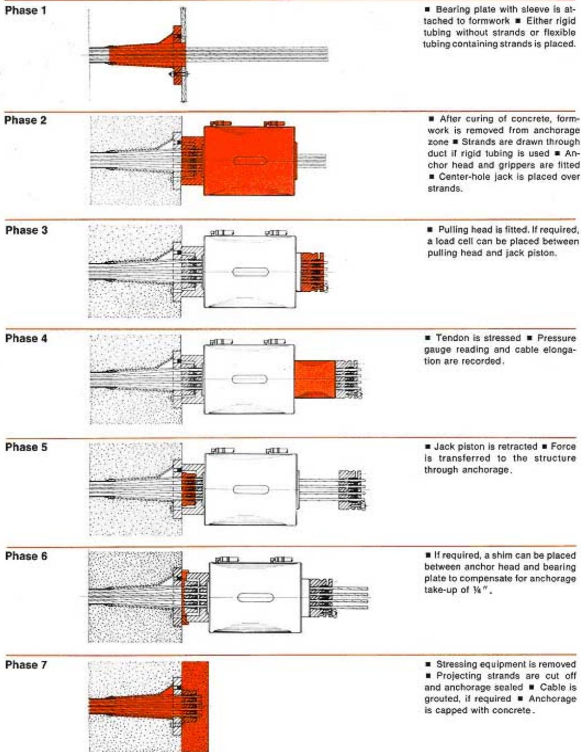
Figure 8-3 – The Complete Jacking Sequence.
