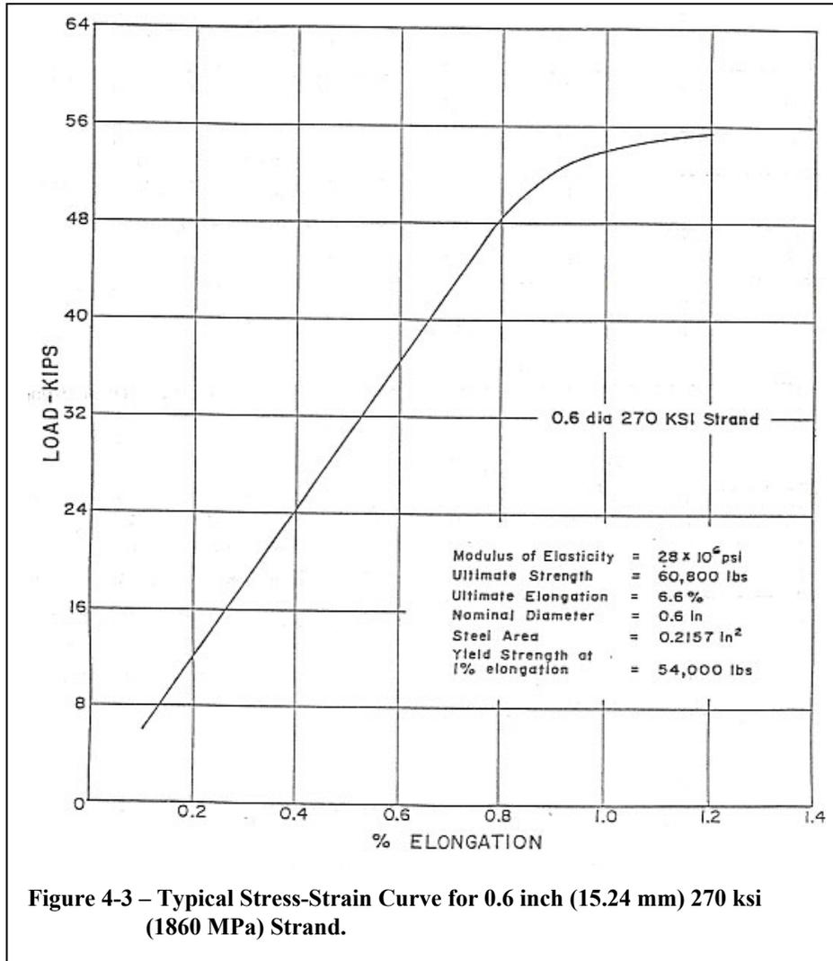
Figure 4-3 – Typical Stress-Strain Curve for 0.6 inch (15.24 mm) 270 ksi (1860 MPa) Strand.
