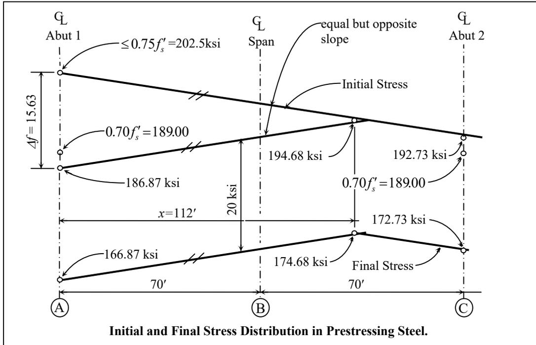
**Part 3:** Final working force at the centerline of span.
