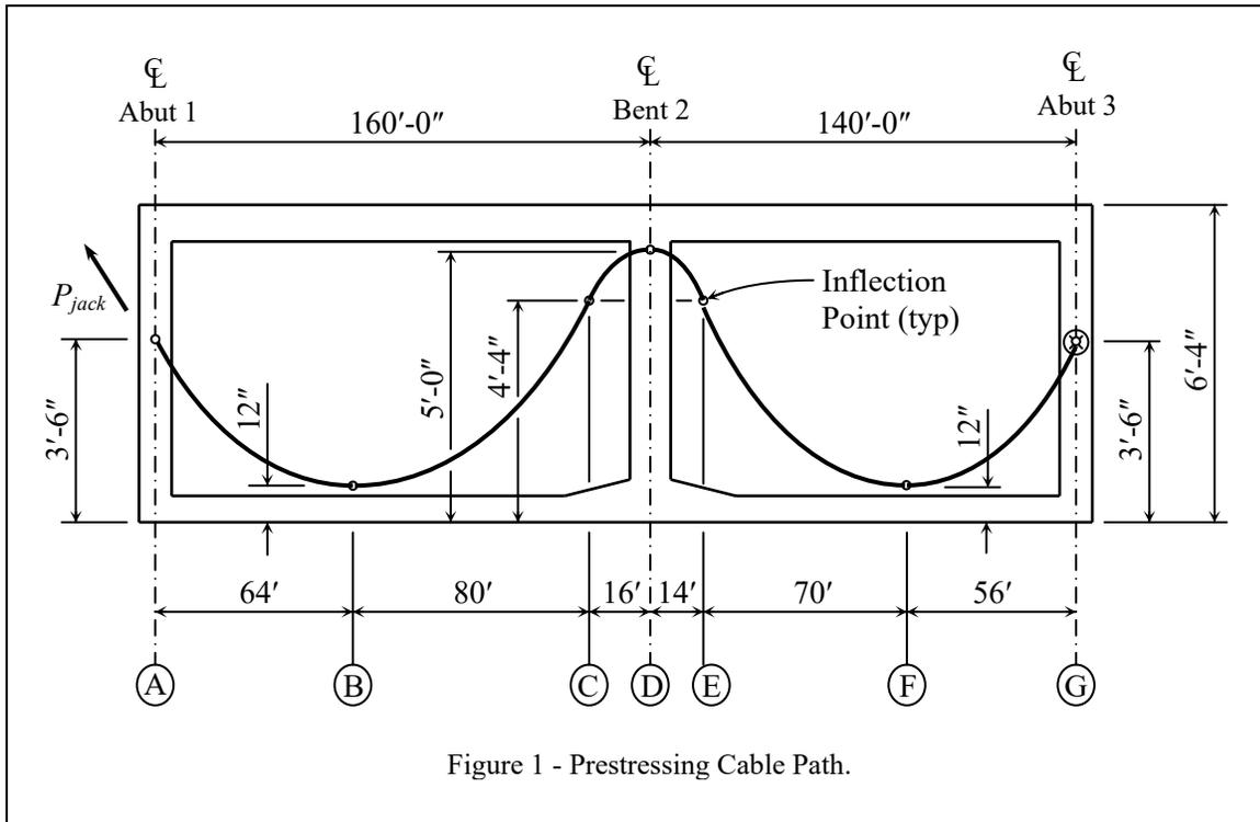
Figure 1 - Prestressing Cable Path.
