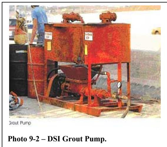
Photo 9-2 – DSI Grout Pump.
