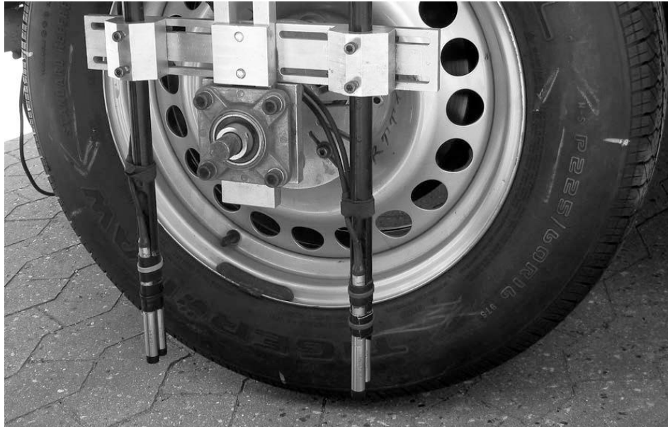
Figure 5-4: Close up of dual probe vertical OBSI setup (shown without required windscreens)
