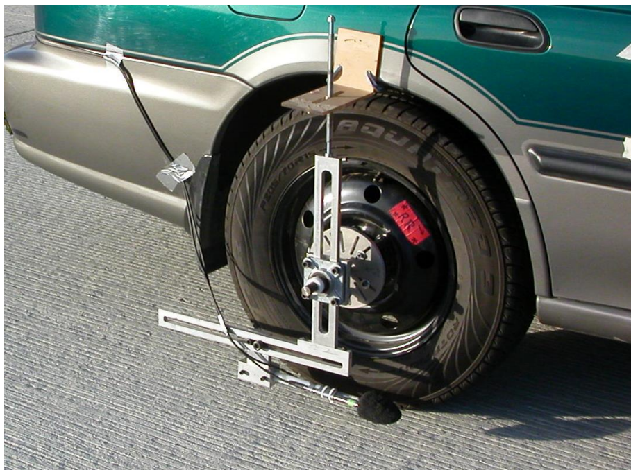
Figure 4-3: OBSI application to tire-pavement noise measurement for purposes of quantifying highway pavement performance (California Department of Transportation 2002)
