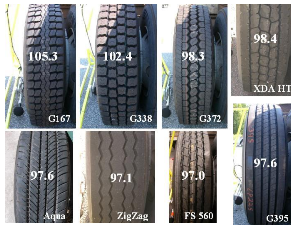
Figure 6-81: Average OBSI levels for truck tires on eight pavements (passenger car Aquatred in lower left).
