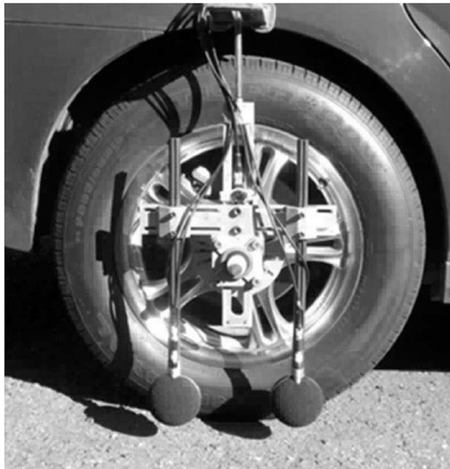
Figure 5-3: Dual probe vertical OBSI setup
