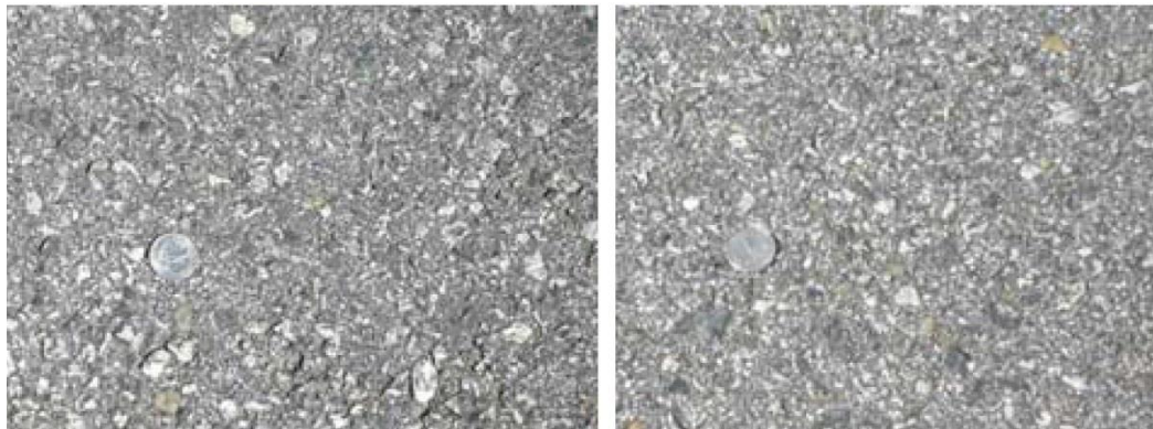
Figure 6-59: Photographs of DGAC pavement at Section 1 (left) and BWC Section 5 (right) in 2008
