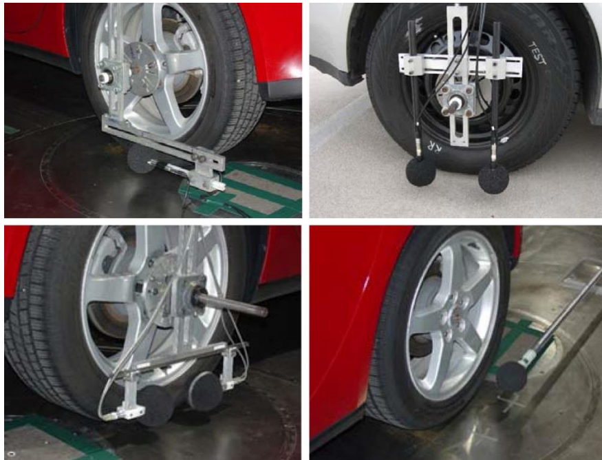
Figure 4-8: Wind tunnel SI probe configurations Upper left: Horizontal Single Probe with Windscreen Upper right: Vertical Dual Probe with Windscreen (On Road) Lower left: Horizontal Dual Probe with Commercial Windscreen Lower right: Probe holder ('ideal fixture') in the trailing edge position
