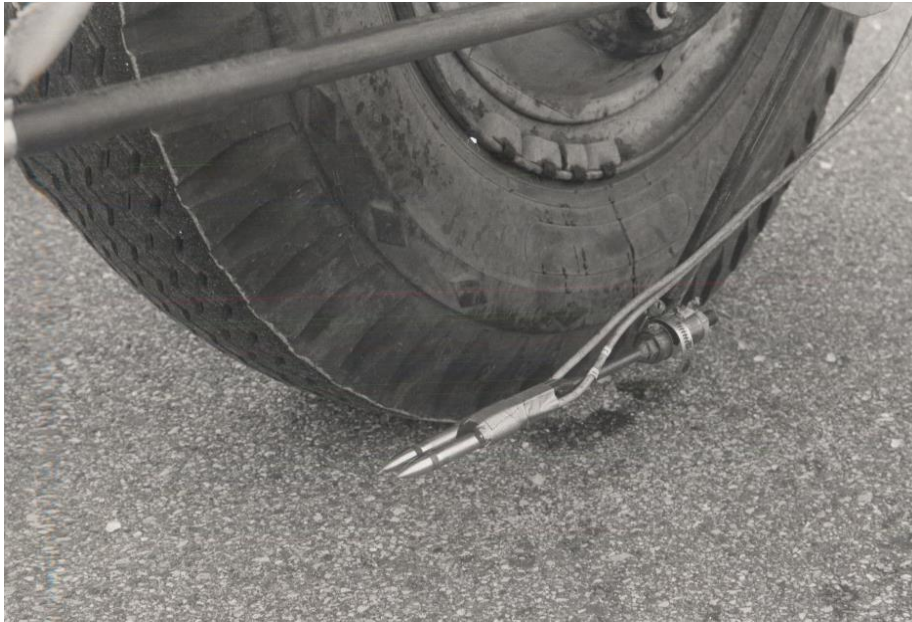
Figure 4-1: First application of OBSI to tire-pavement noise measurement, as used for truck noise source identification at GM
