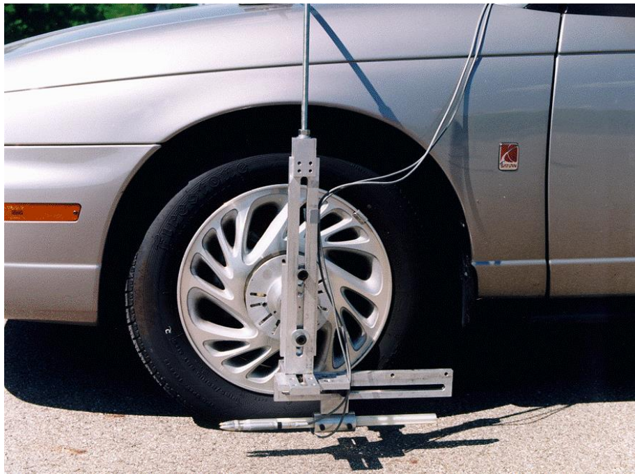
Figure 4-2: OBSI application to tire-pavement noise measurement on passenger cars at GM
