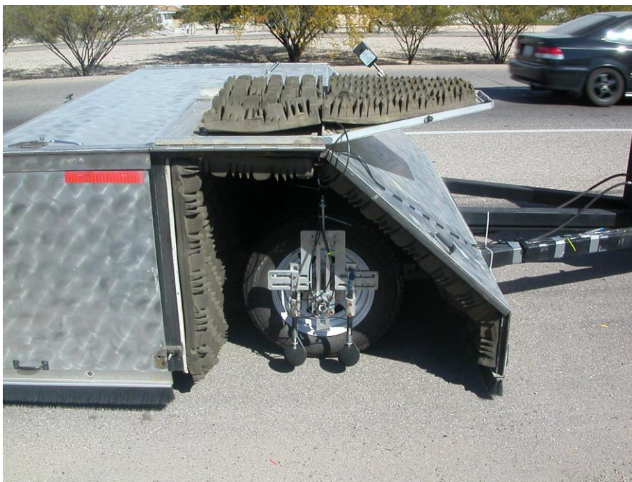
Figure 4-4: First application of dual probe OBSI method for measuring tire-pavement noise on a CPX trailer (Arizona Department of Transportation 2003)
