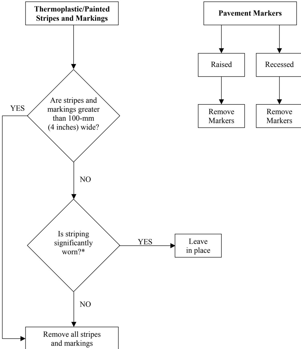
\* Striping has lost retroreflective properties and approximately 50% of pavement is exposed.
