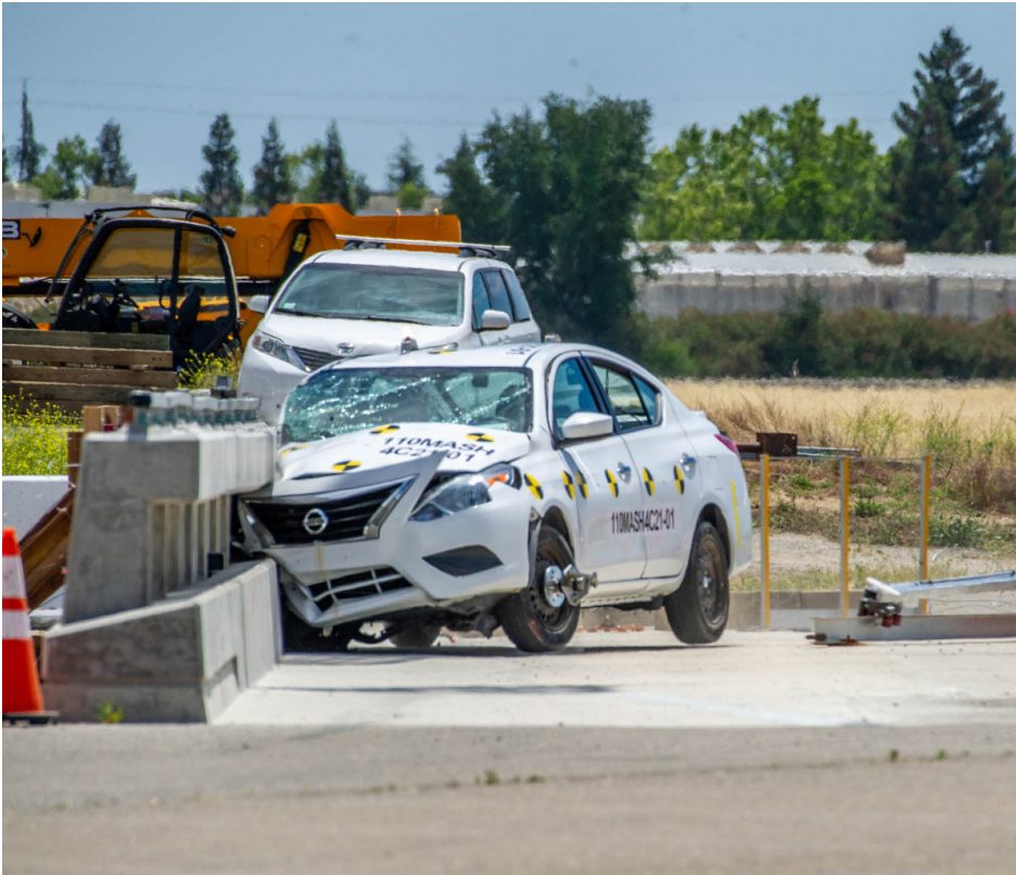
A passenger car crash test on the new Type 86H Concrete Barrier Rail.
