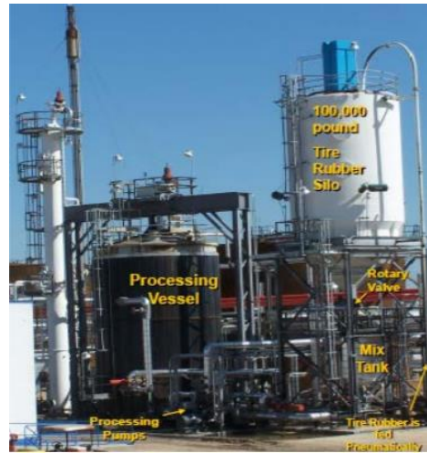
Terminal Blending Process for Rubberized Asphalt
